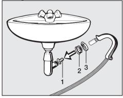
If this nut has a flat disc sealing it you should take the disc out first. Important: if this nut has a washer or seal in it this must not be removed!
